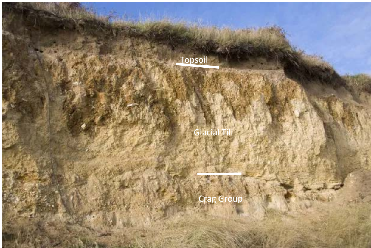
Figure 2. Coastal Cliff at Thorpeness with interpreted lithology. Credit UK Fossils Network website, https://ukfossils.co.uk/dscf4529/ . Annotated by Riggall & Associates
